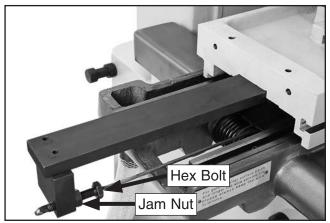
Figure 21. Cable attached to cable bracket.
